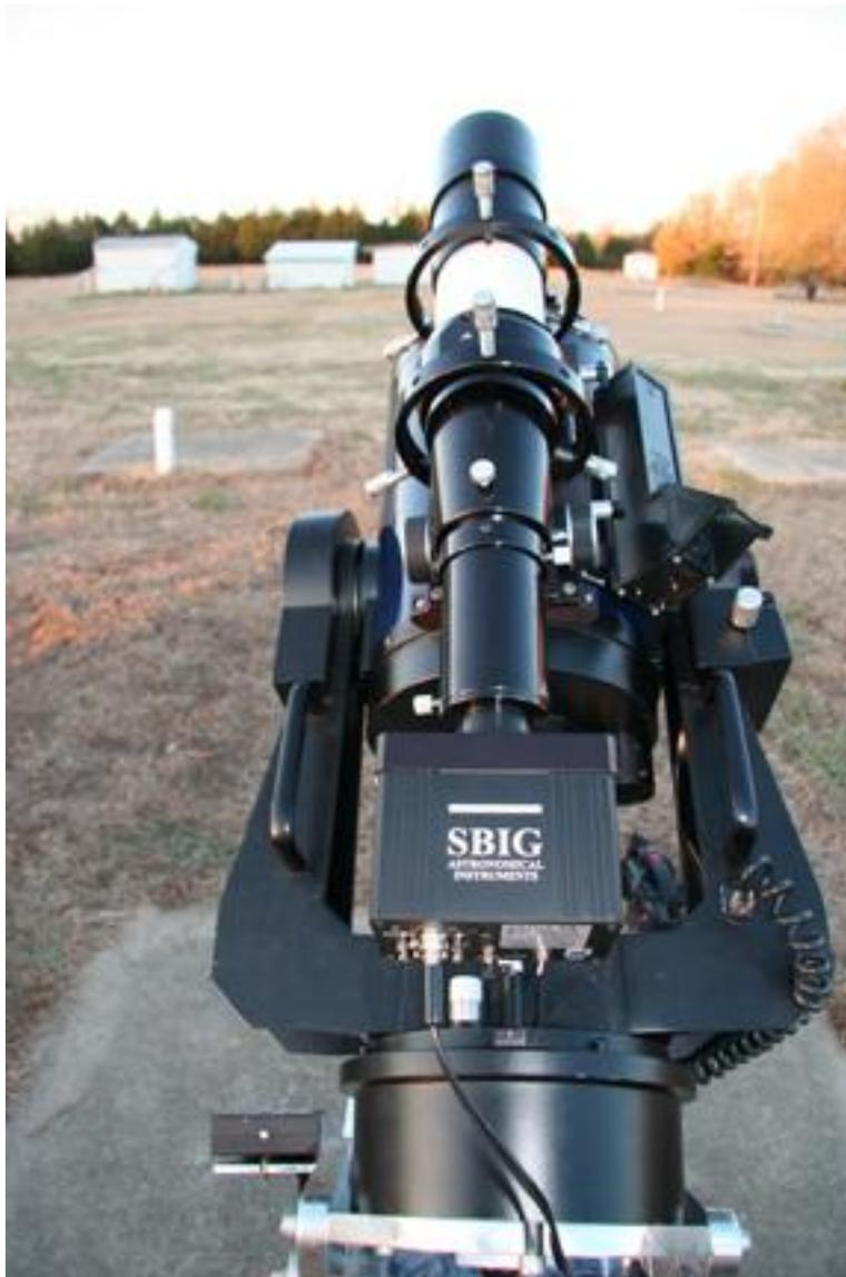
Picture 6: SG-4 attached to a guide scope
