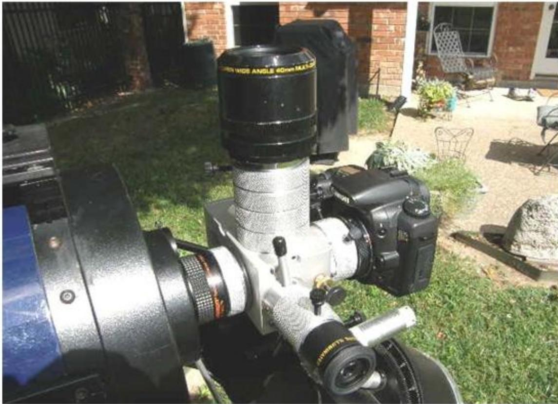
Picture 5: Off-axis guider and equipment
